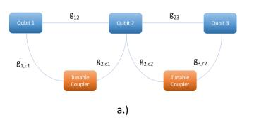
a.) A simplified circuit diagram for our proposed system. b.) A fidelity chart showing the overlap between the ideal Toffoli states and the measured Toffoli states. This shows an overall fidelity of >97% and a gate time of ~700ns.
